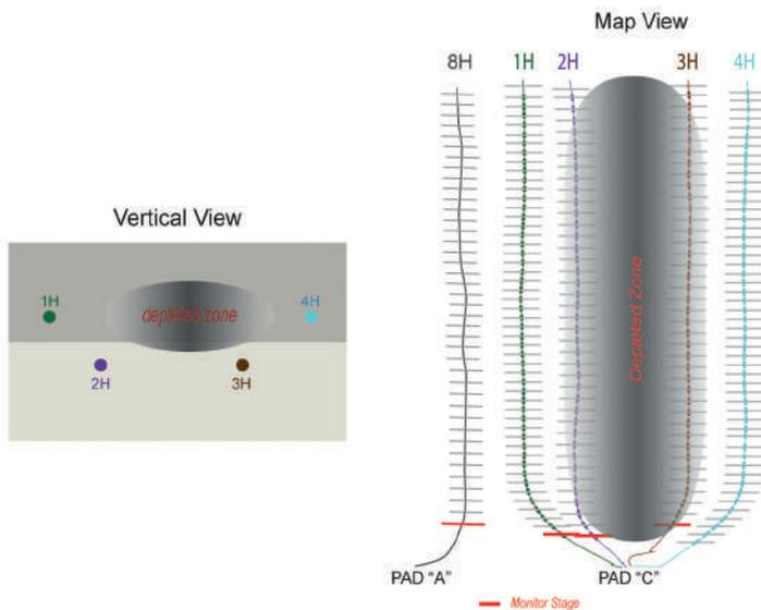
**Figure 1.** Four-well pad, Bakken. This is the vertical view and map view of the four wells on pad C in the Bakken case study.
