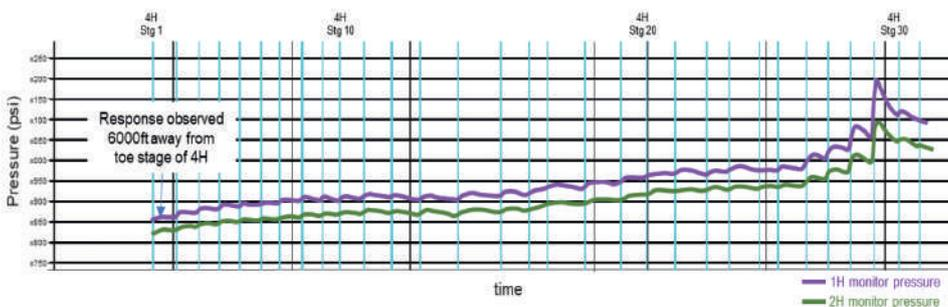
**Figure 3.** Monitored well pressure data. The pressure recorded on wells 1H and 2H shows a pressure response 6000 ft from a stage being fractured on well 4H. The well 4H fractures are pressurizing the depleted zone. With this information, the operator can make treatment design changes to prevent fractures extending into the depleted zone.
