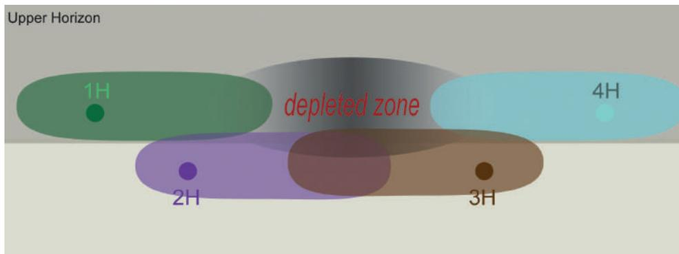
**Figure 2.** Fracture geometry. This is a vertical view showing the heel stages' average fracture geometry. Significant asymmetry observed on the pad's four wells documents that the depletion zone extends into the lower horizon.
